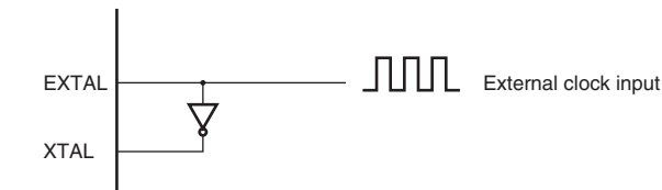
(b) Example of external clock input when an inverted clock is input to XTAL pin
