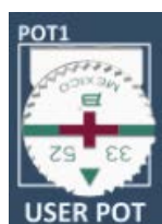
Figure 27. User Potentiometer on Evaluation Kit Board (Top)
