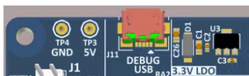
Figure 7. USB Debug Connector (J11), TP3, and TP4 on the Evaluation Kit Board
