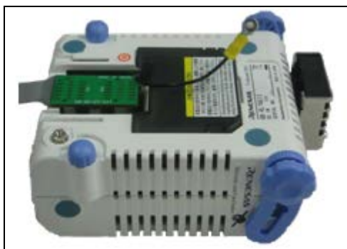
Figure 2-7. Connect the QB-RL78G1F to the probe
