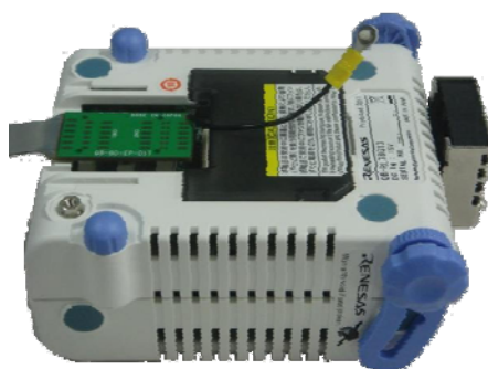
Figure 2-7 Connect the QB-RL78L12 to the probe
