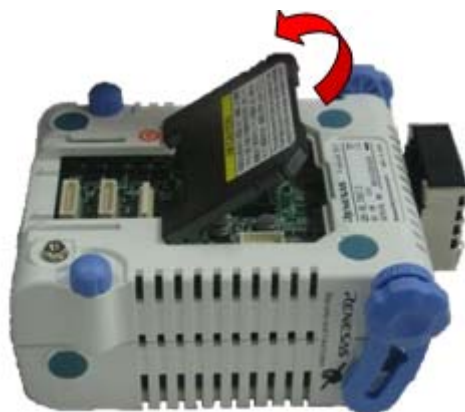
Figure 2-1. Acrylic Board Removal Method
