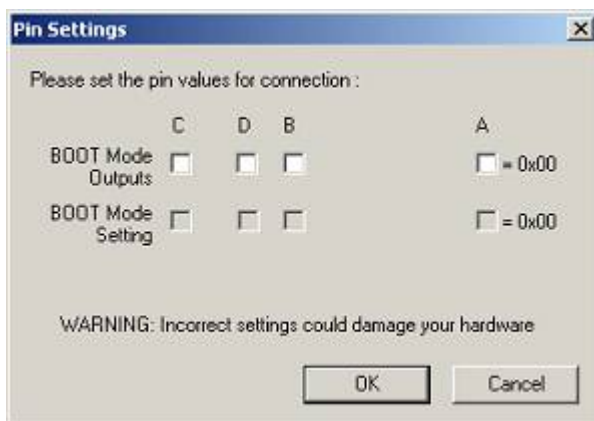
Figure 3-22 E8Direct Generic Device Pin Settings
