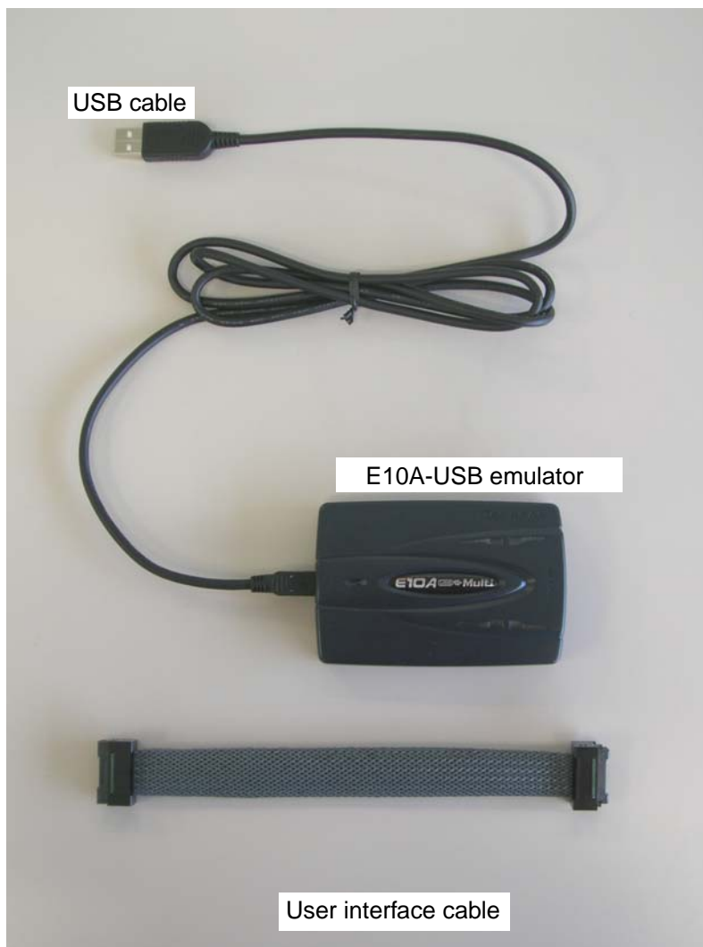
Figure 3.2 Emulator Hardware Configuration (when the 38-pin Type Cable is Used)
