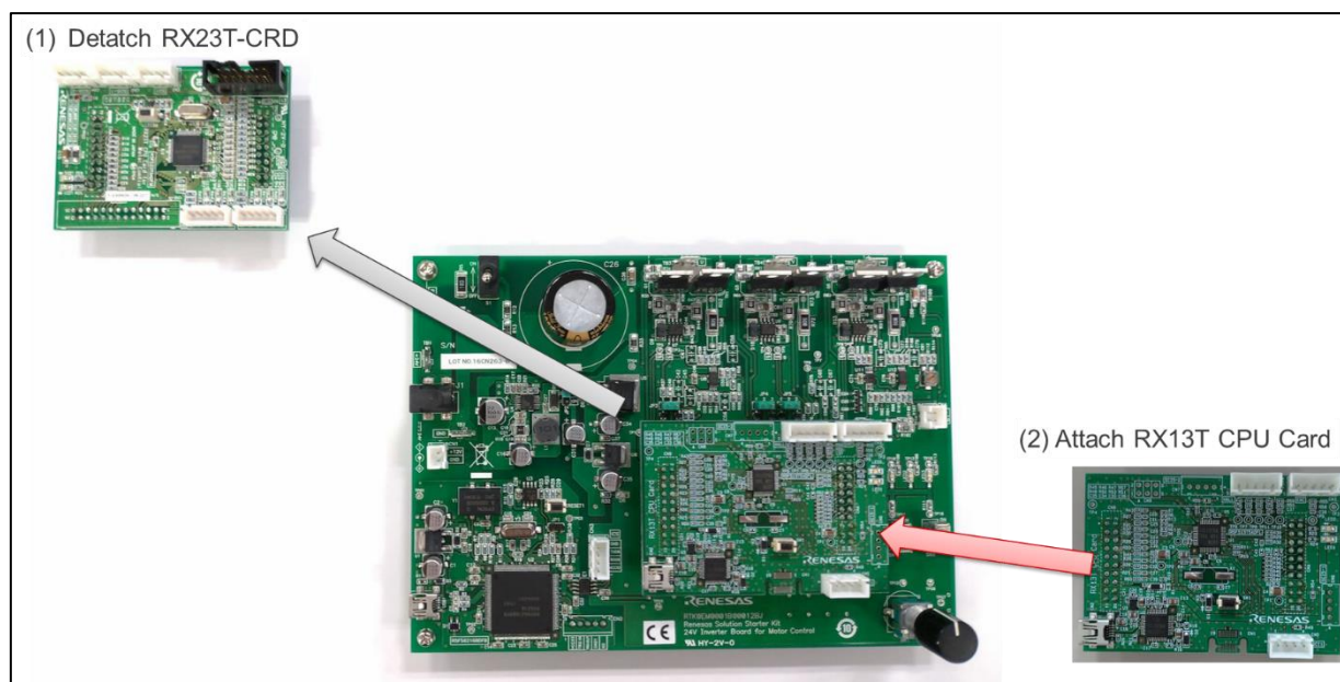
Figure 4-1 CPU card replacement
