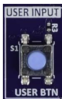
Figure 16. User Switch (S1) on Target Board
