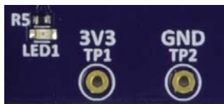
Figure 7. TP1, TP2 and LED1 on Target Board
