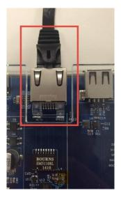
4) Connect the other end of the Ethernet cable to the PoE supply and plug in the power supply.
