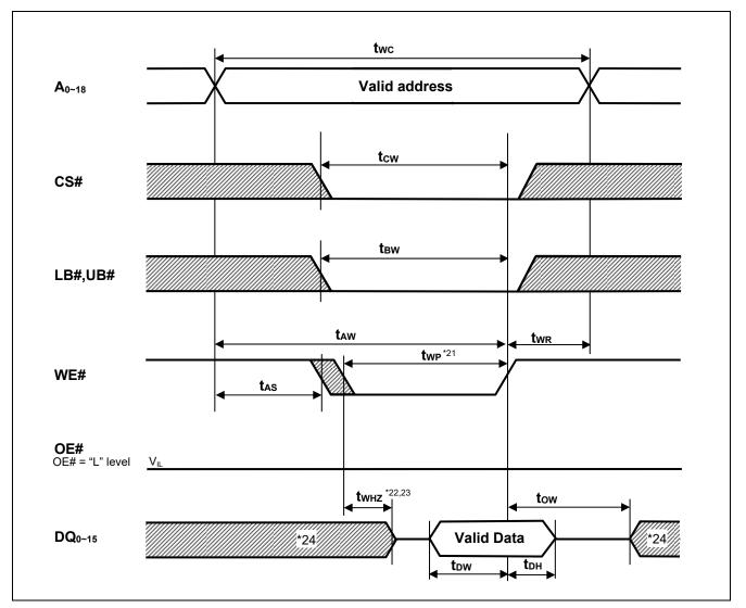
Note 21.  $t_{WP}$  is the interval between write start and write end.
