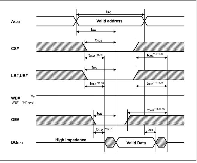
Note 14. t<sub>CHZ</sub>, t<sub>BHZ</sub> and t<sub>OHZ</sub> are defined as the time when the DQ pins enter a high-impedance state and are not referred to the DQ levels.
