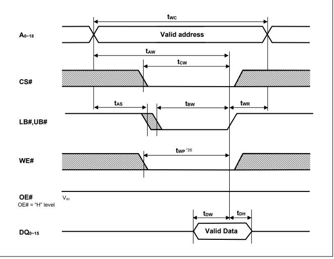
Note 26. twp is the interval between write start and write end.
