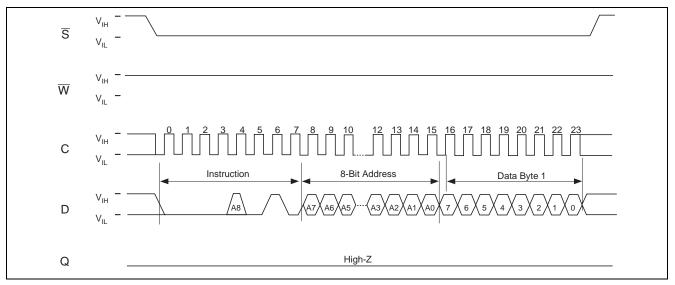
Note: 1. Depending on the memory size, as shown in Address Range Bits table, the most significant address bit is don't care.
