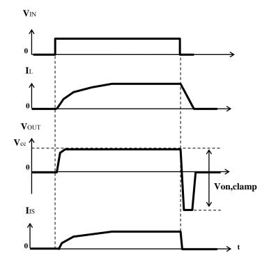
The dynamic clamp circuit works only when the inductive load is switched off. When the inductive load is switched off, the voltage of OUT falls below 0V. The gate voltage of SW1 is then nearly equal to GND. Next, the voltage at the source of SW1 (= gate of output MOS) falls below the GND voltage.
