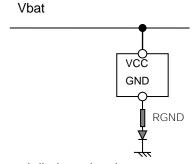
External diode and resistor are recommended in order to prevent reverse current toward control logic part at reverse battery condition and limit the current through  $ZD_{AZ}$  at load dump condition.  $100\Omega$  is recommended as RGND.
