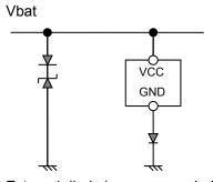
External diode is recommended in order to prevent reverse current toward control logic part at reverse battery condition.
