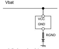
External diode and resistor are recommended in order to prevent reverse current toward control logic part at reverse battery condition and limit the current through  $ZD_{AZ}$  at load dump condition.  $100\Omega$  is recommended as RGND.
