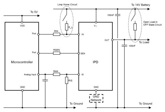
RIN, RSEN, RAN values are in range of 2k to  $50k\Omega$  depending microcontroller while R\_L value is typically  $4k\Omega$ .
