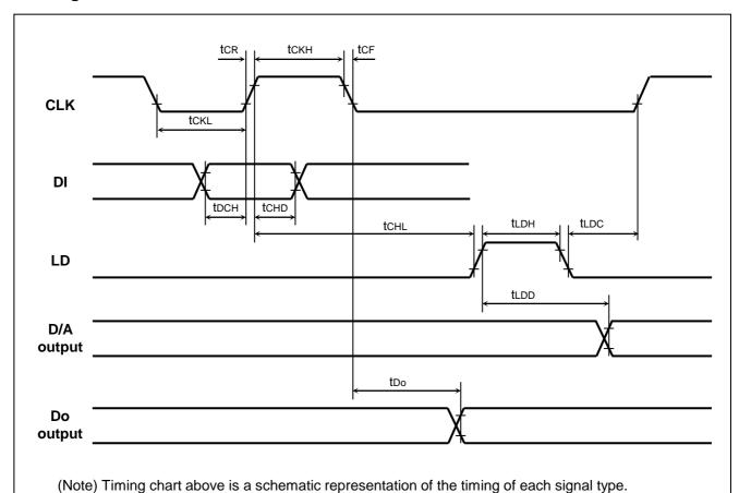
CLK signal input is High or Low regardless, LD signal High input is enabled.
