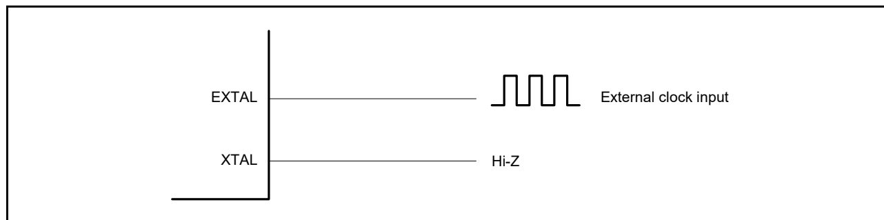
Figure 8.5 Equivalent circuit for external clock
