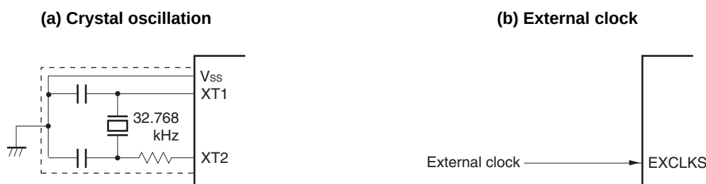
Figure 5-21. Example of External Circuit of XT1 Oscillator
