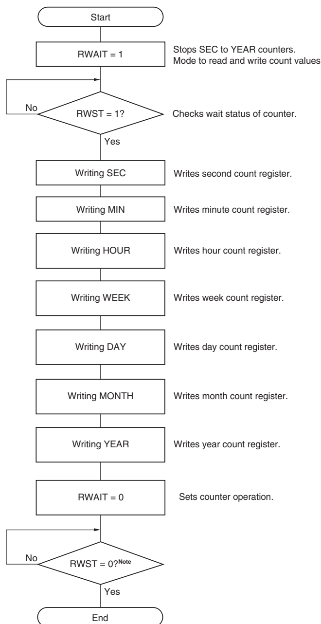
Figure 9-24. Procedure for Writing Real-time Clock
