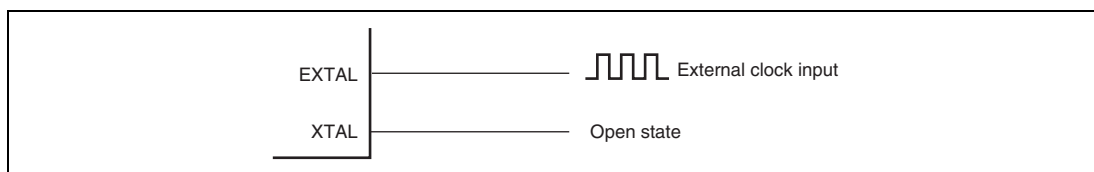
Figure 4.4 Example of External Clock Connection
