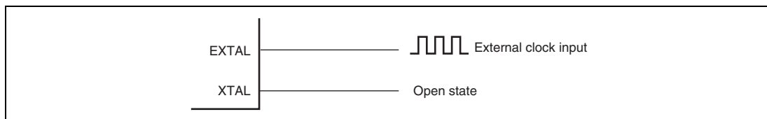
Figure 4.4 Example of External Clock Connection
