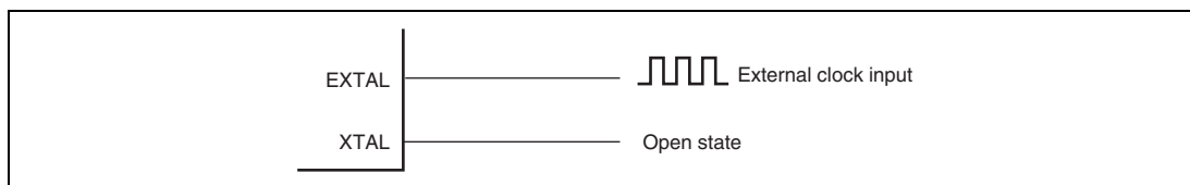
Figure 4.4 Example of External Clock Connection
