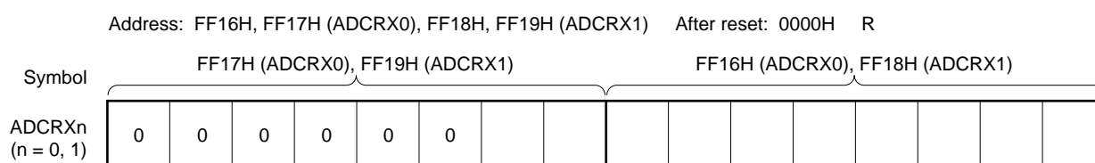
Figure 11-8. Format of 10-Bit A/D Conversion Result Register for TMXn Synchronization (ADCRXn)
