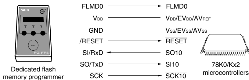
Figure 27-4. Communication with Dedicated Flash memory programmer (CSI10)
