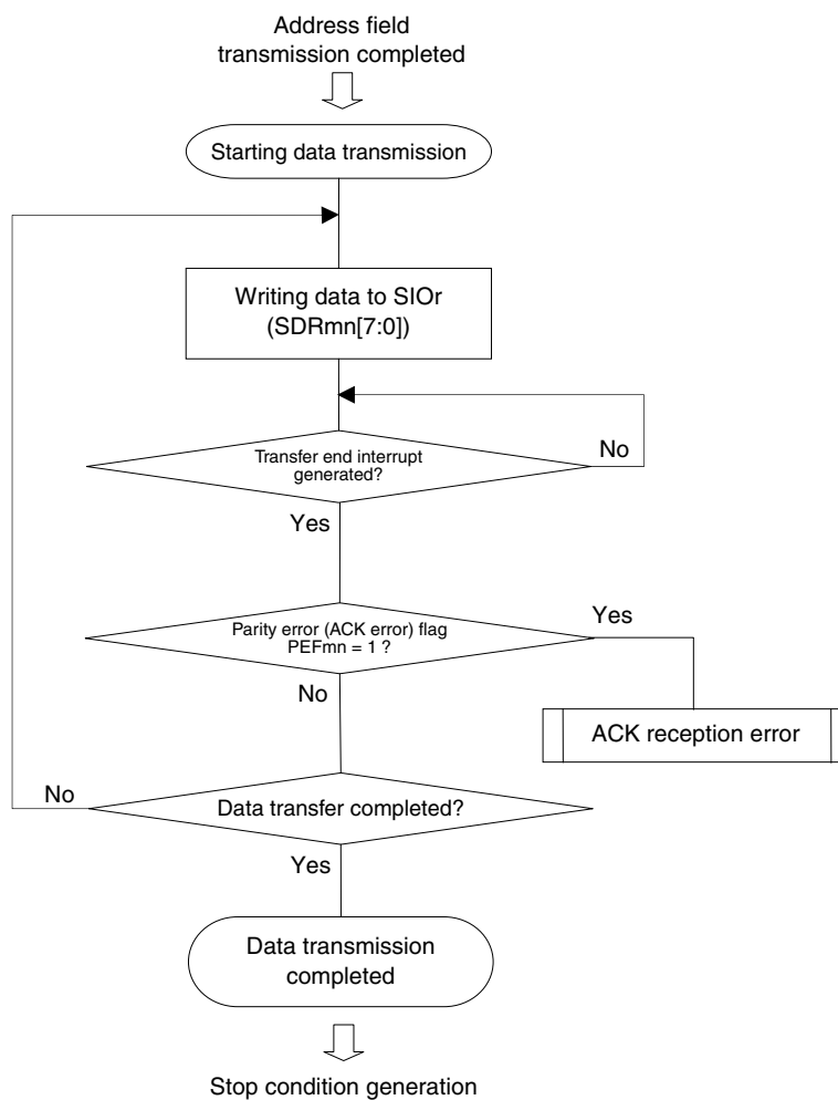
Figure 14-94. Flowchart of Data Transmission
