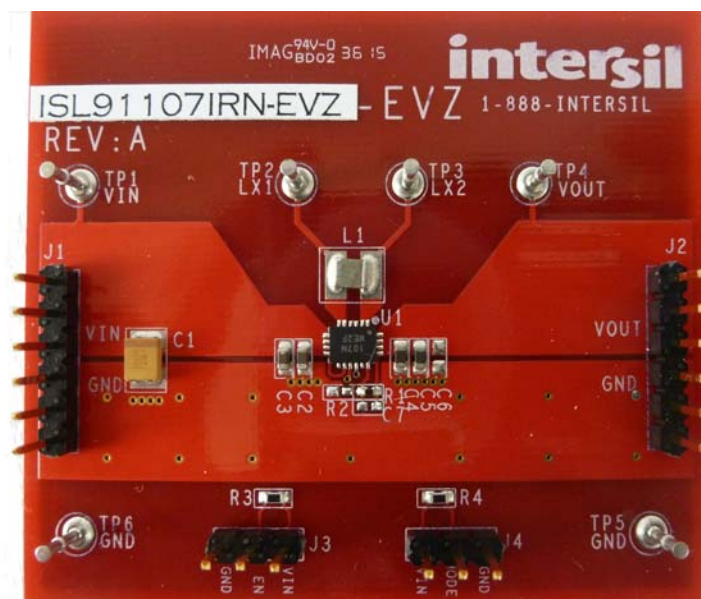
FIGURE 5. ISL91107IRN-EVZ TOP VIEW
