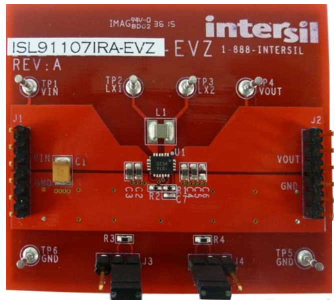
FIGURE 4. ISL91107IRA-EVZ TOP VIEW
