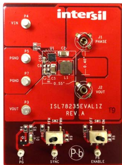
FIGURE 1. ISL78235EVAL1Z EVALUATION BOARD PHOTO
