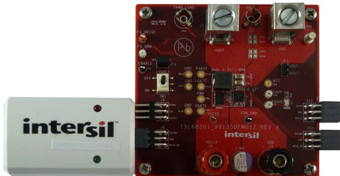
FIGURE 5. ISL68201-99135DEMO1Z DEMONSTRATION KIT SETUP
