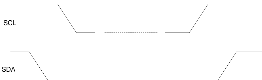
Figure 25: Timing of 2-WIRE START and STOP Condition
