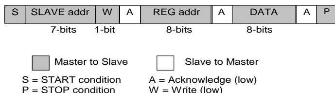
Figure 24: I 2 C Byte Write (SDA line)
