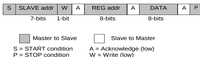
Figure 27. I 2 C byte write (SDA signal)
