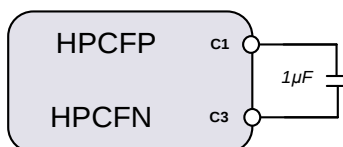
Figure 41. Charge pump flying capacitor
