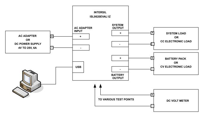
FIGURE 1. ISL9520EVAL1Z HARDWARE CONNECTION DIAGRAM
