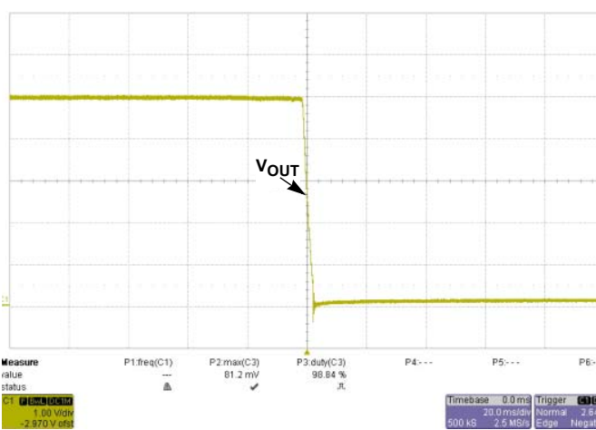
FIGURE 8. SHUT-DOWN AT V_{IN} = 36V @ I_O = 0A
