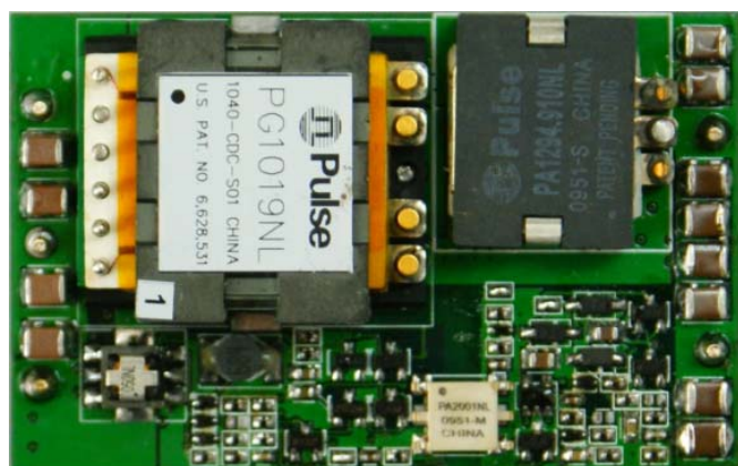
FIGURE 1. TOP VIEW OF ISL6726EVAL1Z (ACTUAL SIZE: 40x60x16mm)
