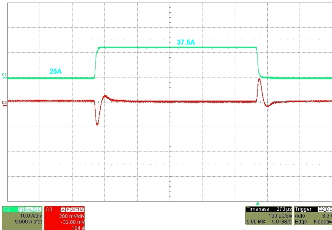
FIGURE 24. STEP LOAD: 25A TO 37.5A (12.5A DELTA)
