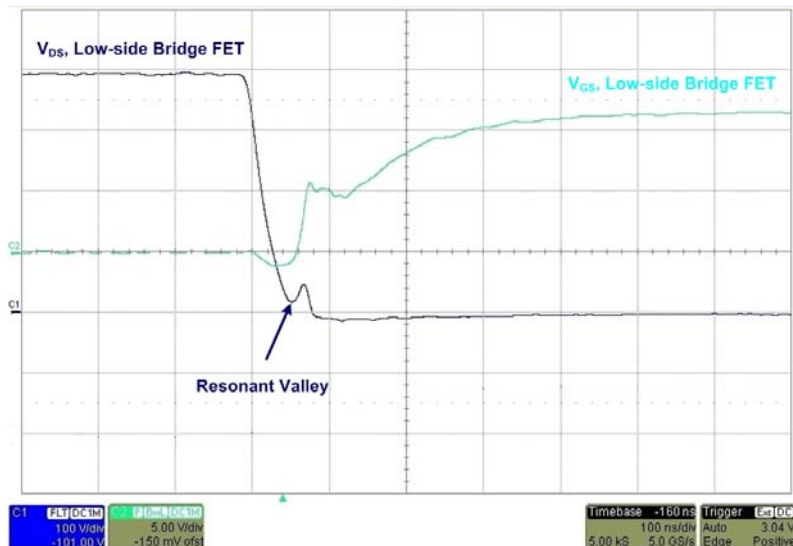
FIGURE 21. RESONANT SWITCHING WITH 100% (50A) LOAD
