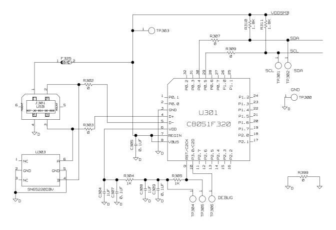
FIGURE 11. ISL88731(C)EVAL2Z SCHEMATIC (USB - SMBUS INTERFACE)
