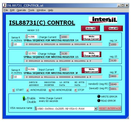
FIGURE 5. ISL88731(C)EVAL2Z CONTROL SOFTWARE SCREEN SHOT
