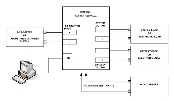
FIGURE 1. ISL88731(C)EVAL2Z HARDWARE CONNECTION DIAGRAM
