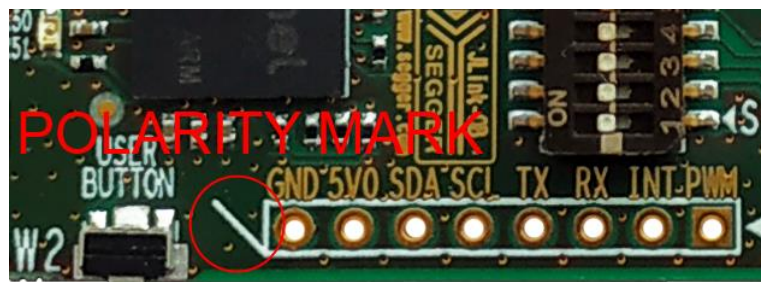
Figure 18. Guides for proper mikroBus™ click board insertion
