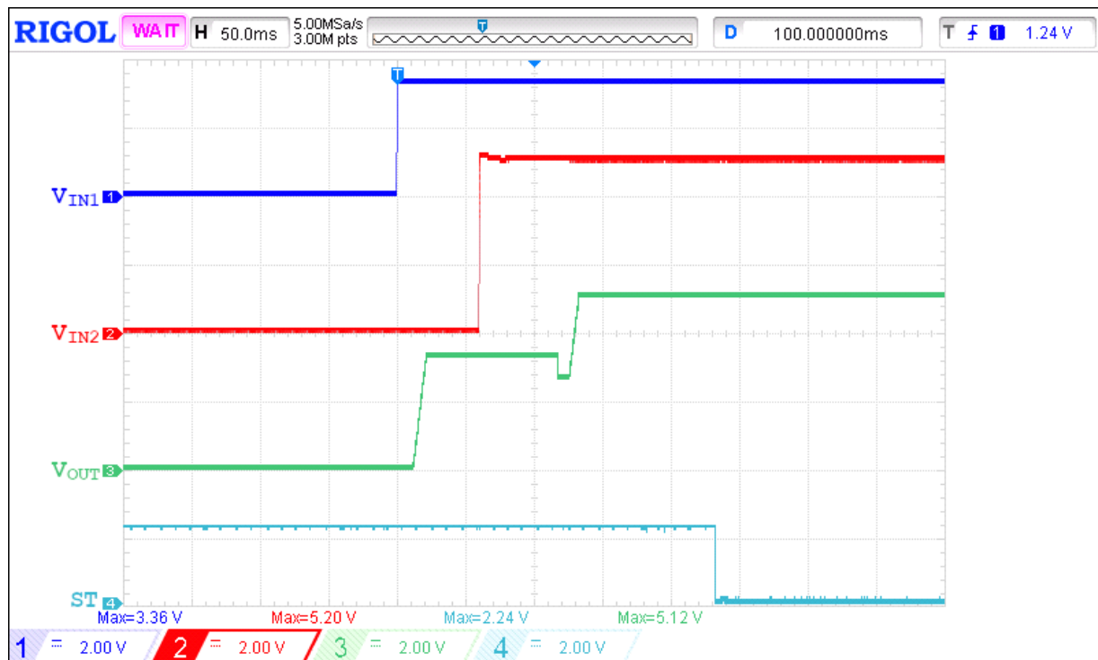
Figure 11. Higher voltage level priority operation waveform for V_{IN1} = 3.3\text{ V} , V_{IN2} = 5\text{ V} , SEL = 0\text{ V} , PR = 0\text{ V} , C_{SS} = 220\text{ nF} , R_{LOAD} = 100\text{ }\Omega , C_{LOAD} = 2\text{ }\mu\text{F}
