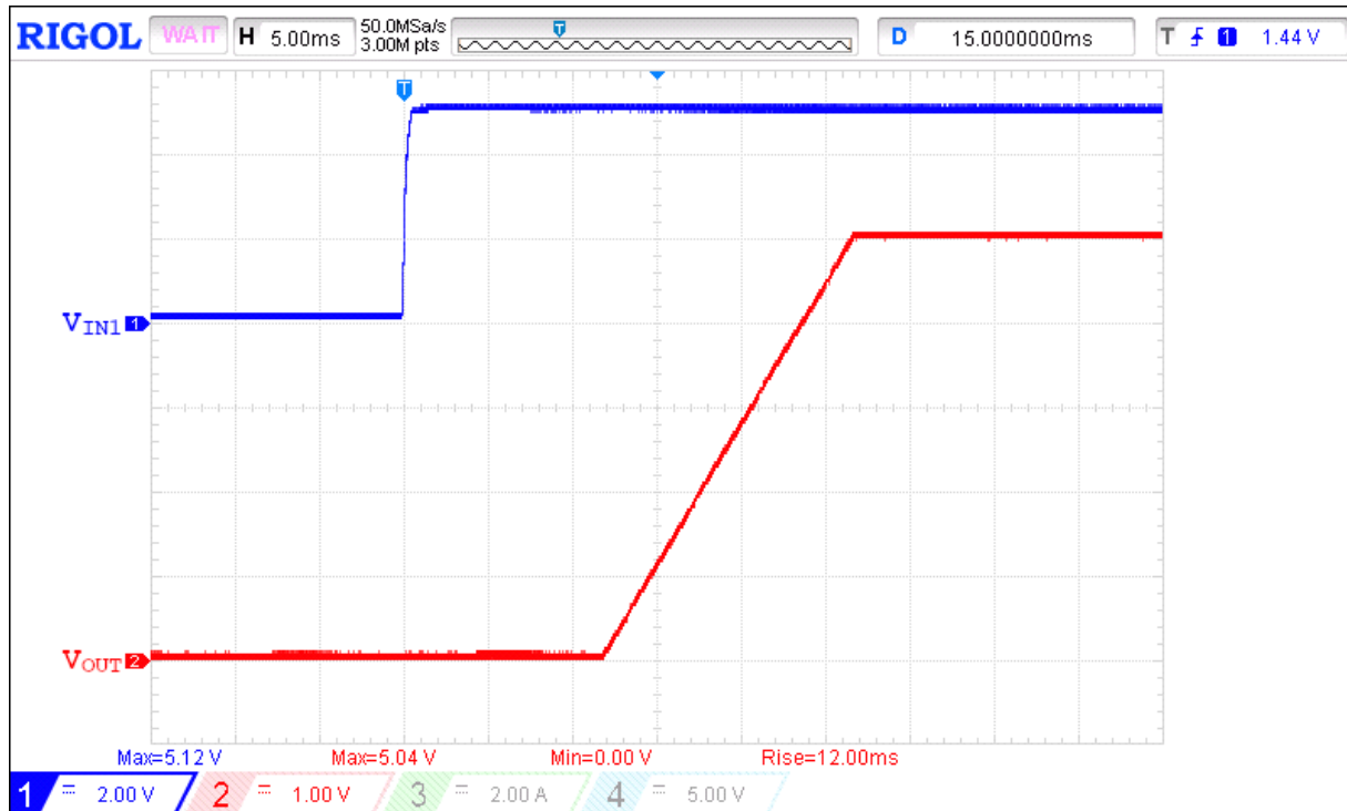
Figure 1. Typical Turn ON operation waveform for V_{IN1} = 5\text{ V} , C_{SS} = 220\text{ nF} , R_{LOAD} = 100\text{ }\Omega , C_{LOAD} = 2\text{ }\mu\text{F}
