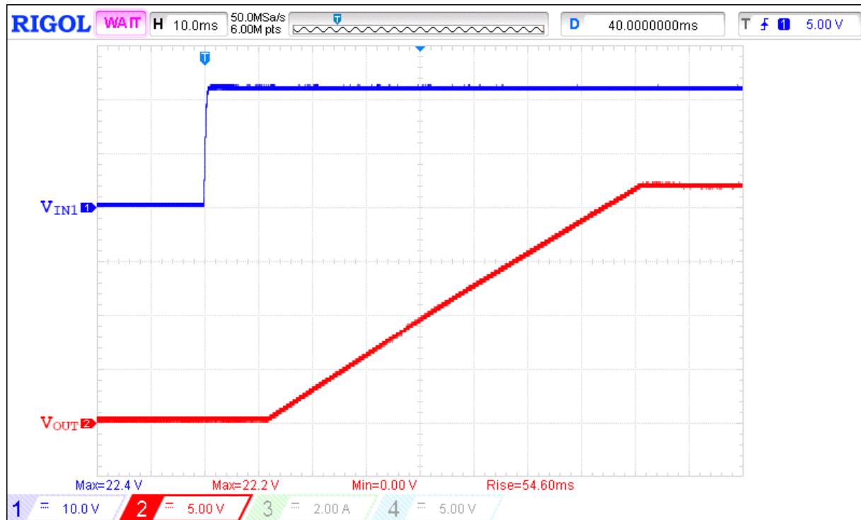
Figure 3. Typical Turn ON operation waveform for V_{IN1} = 22\text{ V} , C_{SS} = 220\text{ nF} , R_{LOAD} = 100\text{ }\Omega , C_{LOAD} = 2\text{ }\mu\text{F}
