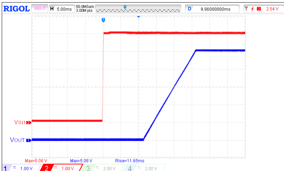
Figure 2. Typical Turn ON operation waveform for V_{IN1} = 5\text{ V} , C_{SS} = 220\text{ nF} , R_{LOAD} = 100\text{ }\Omega , C_{LOAD} = 2\text{ }\mu\text{F}
