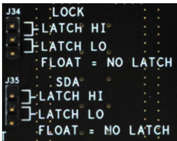
Figure 7. Lock Pin and SDA Pin Latch Control
