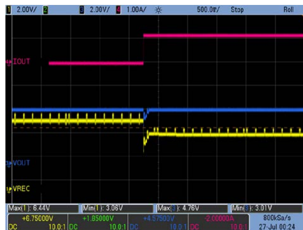
Figure 13. Load Transient: V_{OUT} = 4.5V , 0A \rightarrow 1.2A
