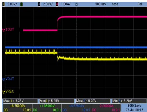
Figure 11. Load Transient: V_{OUT} = 5V , 0A \rightarrow 1.2A
