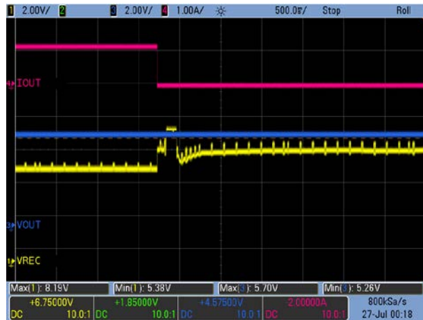
Figure 12. Load Transient: V_{OUT} = 5V , 1.2A \rightarrow 0A
