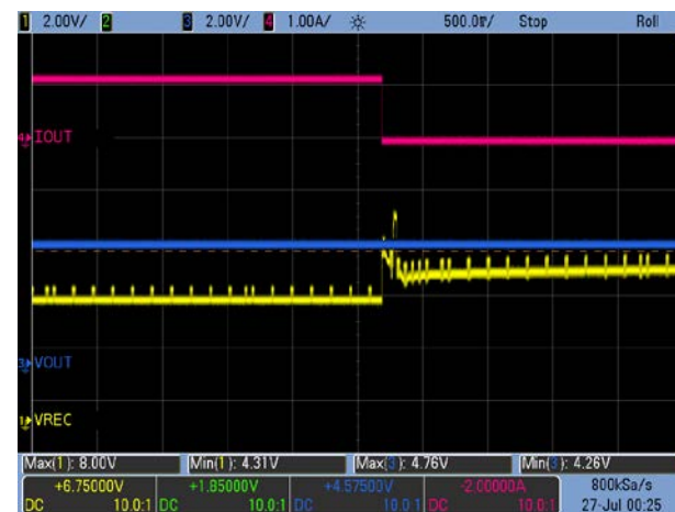
Figure 14. Load Transient: V_{OUT} = 4.5V , 1.2A \rightarrow 0A
