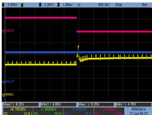
Figure 12. Load Transient: V_{OUT} = 5V , 1.2A \rightarrow 0A
