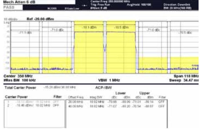
Fig 22. ACLR of 2 carriers LTE (BW=2 x 20 MHz) centered at 350 MHz
