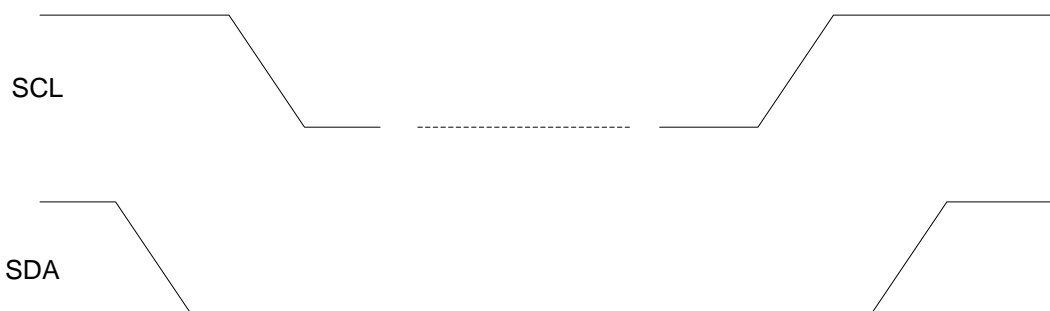
Figure 22: Timing of 2-WIRE START and STOP Condition
