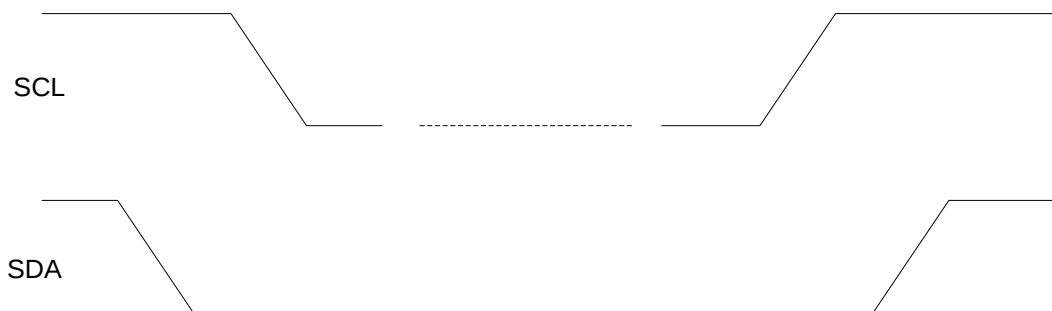
Figure 9: I 2 C START and STOP Condition Timing
