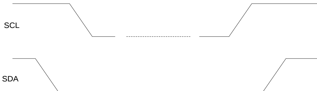
Figure 9: I 2 C START and STOP Condition Timing
