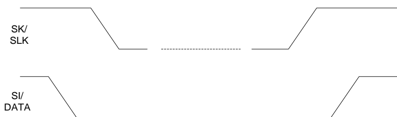
Figure 24: Timing of 2-WIRE START and STOP Condition
