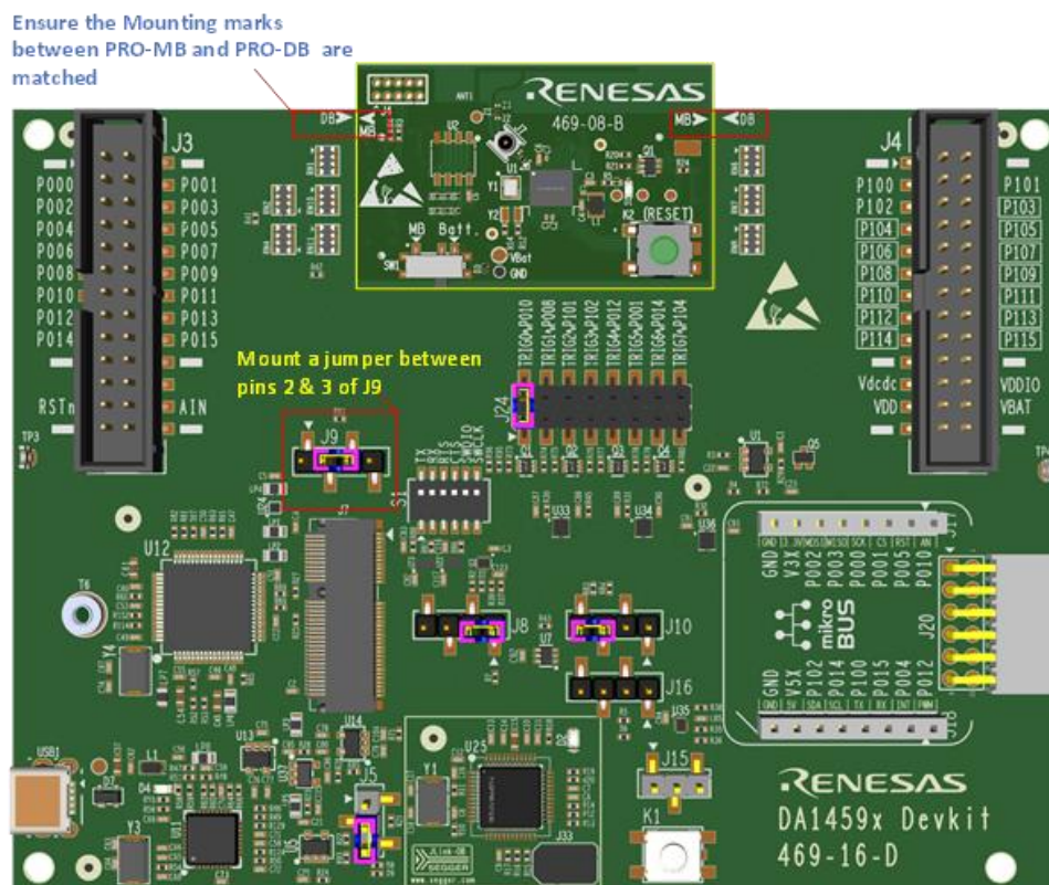
Figure 5. Hardware setup of DA1459x Pro-Devkit without PMM2
