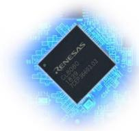
The CL8000 product family is a powerful, highly integrated, Wi-Fi 6 (802.11ax R2) chip family employing a disruptive concurrent dual-band, dual-function, dual transceiver 8T8R flexible MIMO architecture that can drive PHY/Data Link speeds up to 6Gbps for concurrent dual band operation in a single chip.
