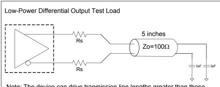
Note: The device can drive tranmission line lengths greater than those allowed by the PCle SIG.
