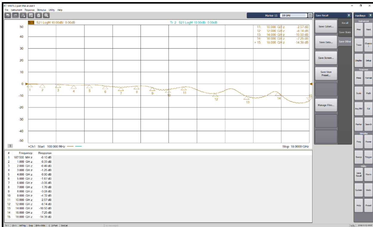
Figure 14. 8V97003 EVB Revision C Transmission Line Loss
