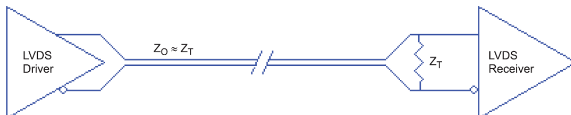
Figure 4. Standard LVDS Termination
