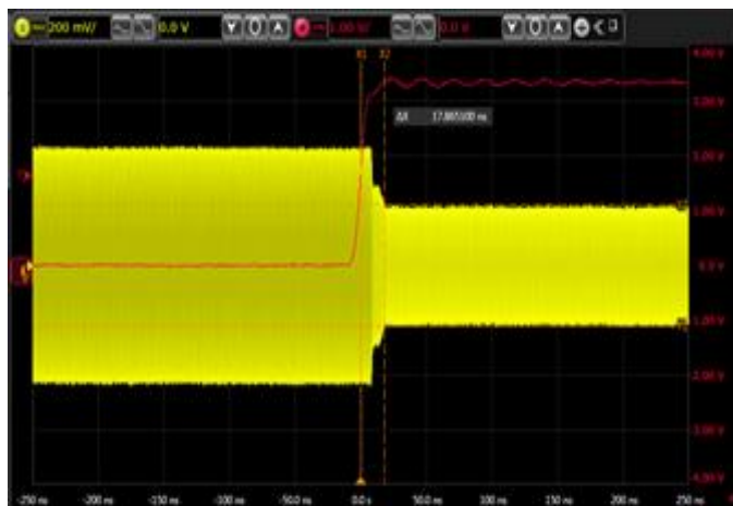
Figure 25. 6dB Gain Reduction Transient Time
