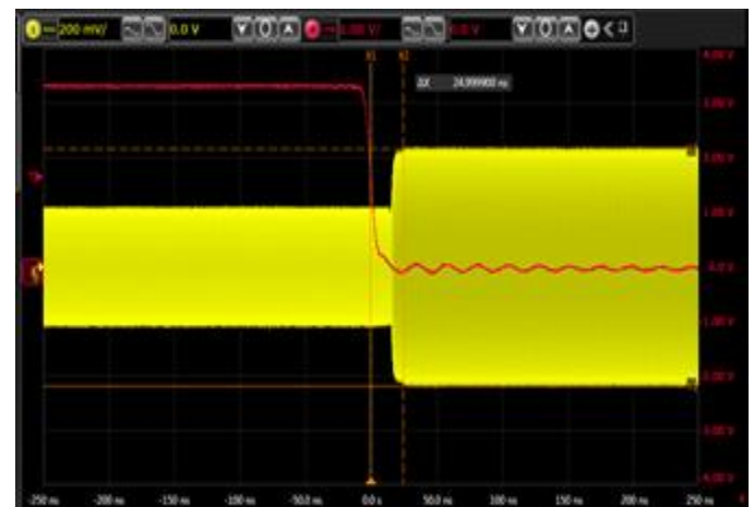
Figure 26. 6dB Gain Increase Transient Time
