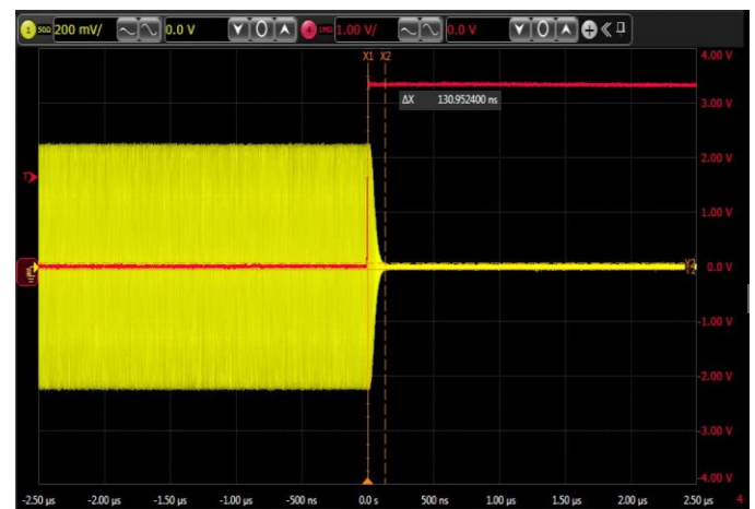
Figure 26. 6dB Gain Increase Transient Time
