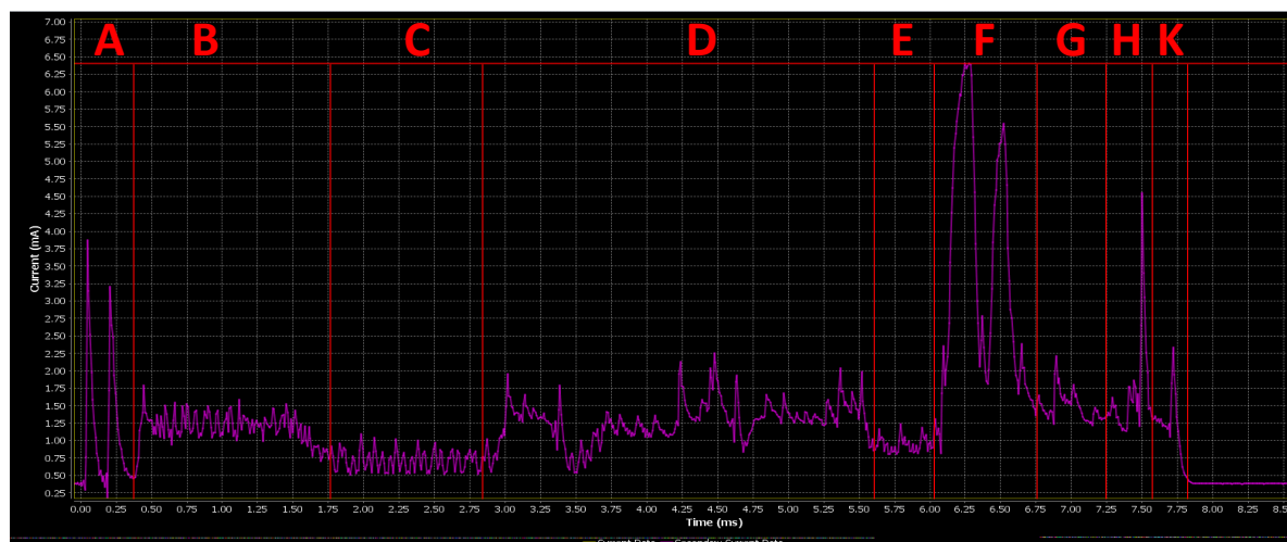
Figure 123: BLE Connection power profile
